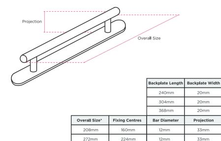
Fixings: Supplied 2 x M4 fixing bolts.
