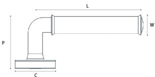
148<sub>mm</sub> 65<sub>mm</sub>  $58 \, \text{mm}$ 25<sub>mm</sub> Length (I) Projection (p) Max Grip Width (w) Rose (c)
